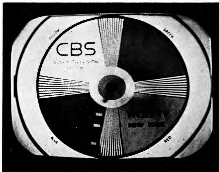
Fig. 9. Test pattern transmitted with 4.5-mc cutoff frequency, uncrispened.
